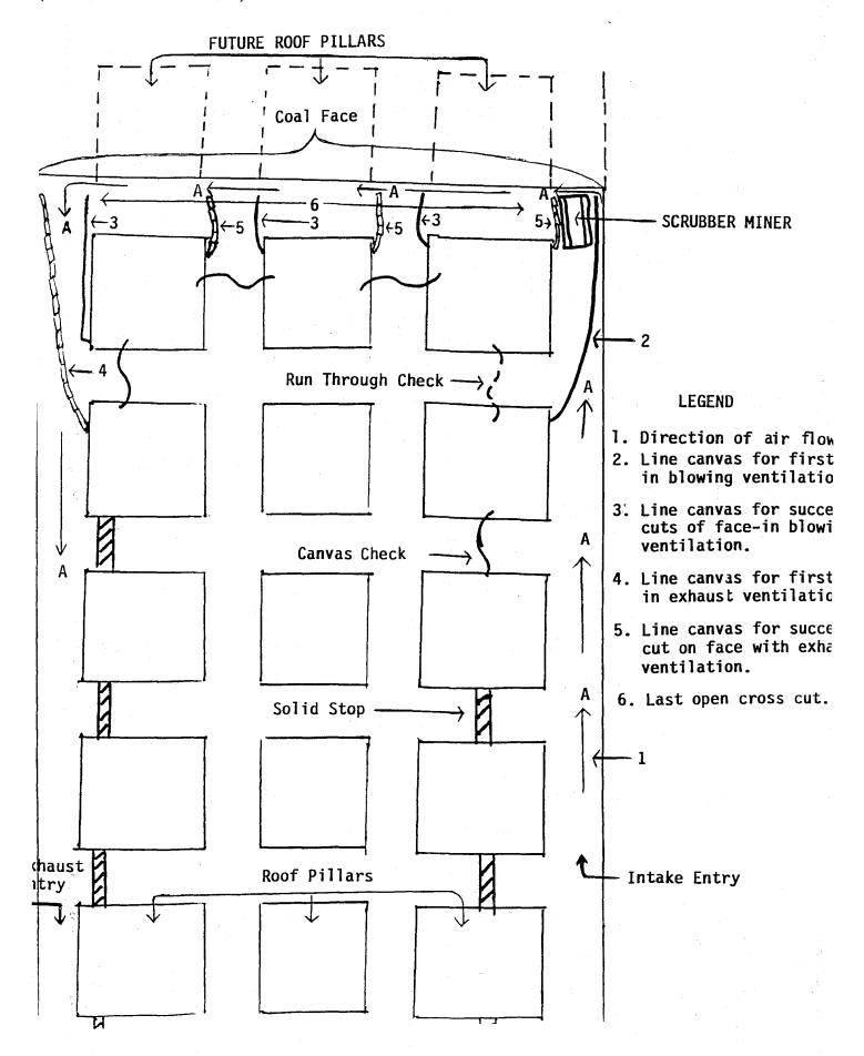
Since no coal is produced in the time a continuous mining machine is moved and the line canvas is reset, and it must be moved more often in an exhaust ventilation operation because of the short cuts, it is obvious from a production standpoint that SM technology is much preferable by mining companies.
